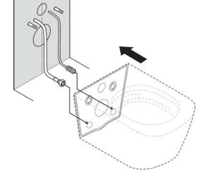
We suggest using the TOTO connecting set SP10695UN for hidden connections WASHLET™ RX, SX GL 2.0, EK 2.0 to prepare the water connection on Geberit frames with empty conduit (located on the left hand side 50 mm from the center of the frame at the same height as the fixation bolts).
