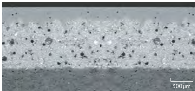
CEFIONTECT toilet micrograph * 1 μm=0.001 mm
